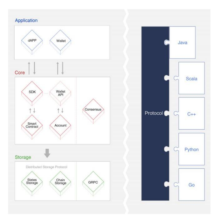
Figure 1: TRON 3-layer Architecture
